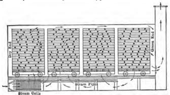
Fig. 94.—Scheme of a progressive kiln operated by natural ventilation. The entering air passes through the heating coils beneath the lumber piles then up through the lumber and out by way of the chimney. Steam may be admitted to raise the humidity.
